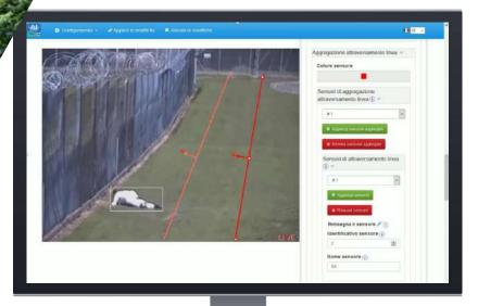
Al-Intrusion is the video analytic module which allows to reveal intrusions in sterile zones and crossing of virtual lines (for instance for the perimetral security of the building).
