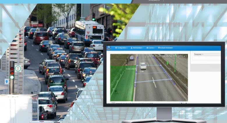
AI-INCIDENT-DEEP is the video analytics solution for traffic monitoring, the smart roads and the smart cities. Thanks to advanced algorithms based on the use of deep neural networks, AI-INCIDENT-DEEP can be used to extract alarmist information relating to the crowding of vehicles on the road.
